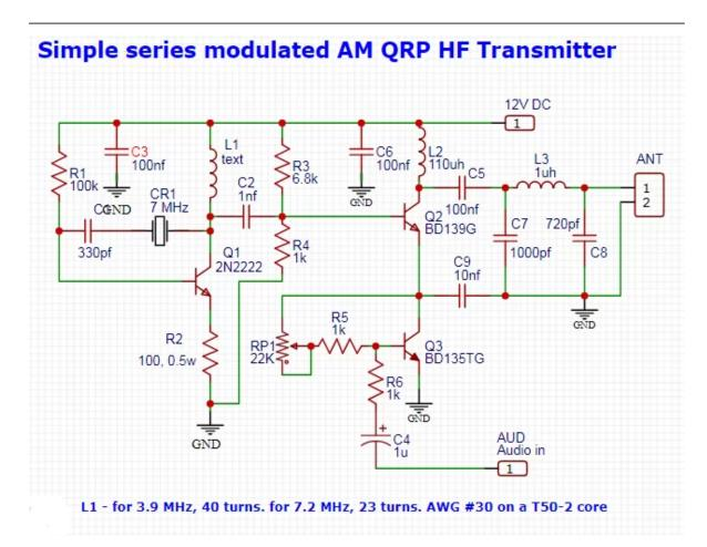
A **simple series modulated AM QRP HF transmitter** is a type of radio transmitter that uses amplitude modulation (AM) to transmit audio signals over a high frequency (HF) radio band. It is designed to be low-power and simple to construct, making it a good choice for beginners or those who want to
