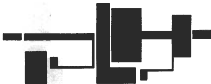
Fig 14—Full-scale PC-board pattern for the broadband 500-mW SD1598 amplifier. Black areas represent unetched copper foil.
